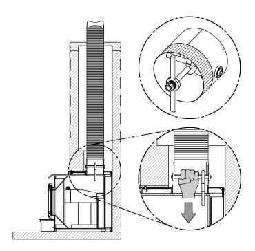
Figure 20: Liner fastening system
