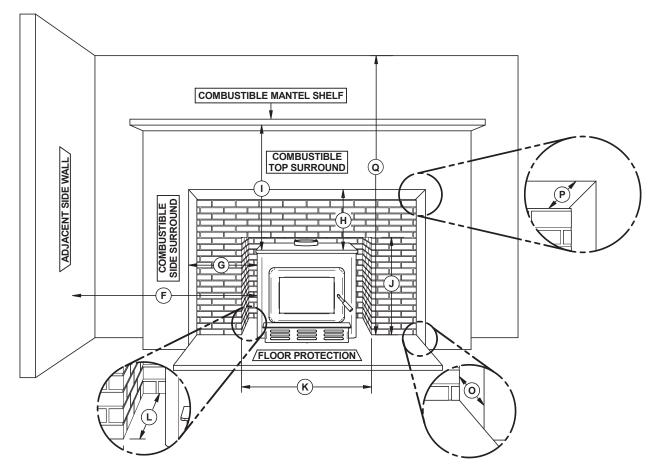
Figure 15: Masonry Opening and Clearances
