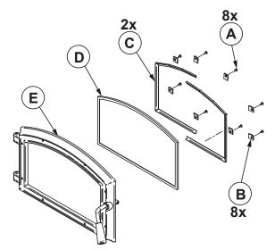
The two main causes of broken door glass are uneven placement in the door and overtightening the retaining screws.
