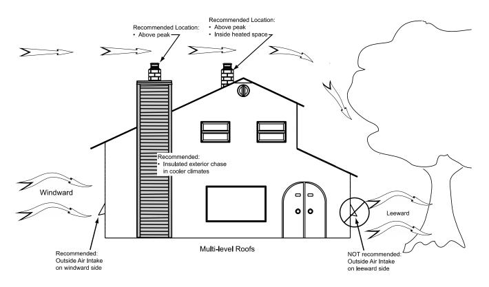
Figure 23: Air supply in conventional houses
