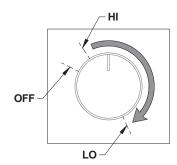
The insert is also equipped with a heat sensor who works with the blower. When the blower is on (position between LO and HI), the thermodisc will start the blower automatically when the insert is hot enough and it will stop it when the insert has cooled down. Therefore, the variable speed control can be left at the desired setting.
