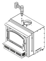
Figure 19: Securing the brackets
