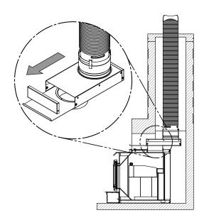
Figure 22: Offset liner adaptor
