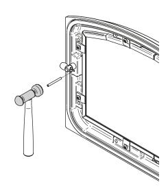
Figure 10: Installing the split pin
