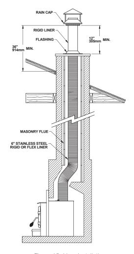
Figure 18: Liner Installation
