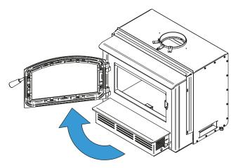
2. Hold the fire screen by the two handles and bring it close to the door opening.
