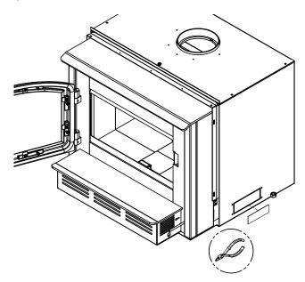
2. Install the fresh air intake adapter **(E)** with four screws **(F)** then secure the flexible pipe<sup>15</sup> **(H)** (not included) to the adapter using one of the pipe clamps **(G)**. Secure the other end of the pipe to the outside wall termination **(J)** using the other pipe clamp. The outside wall termination must be installed outside of the home.
