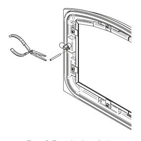
Figure 9: Removing the split pin
